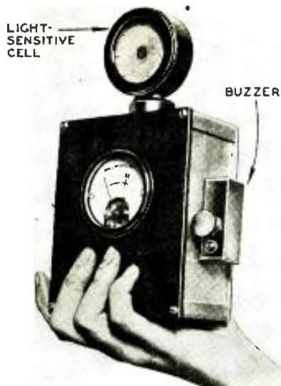
Fig. B The photoelectric guide unit, with its photonic cell on the top and a buzzer on the side.
