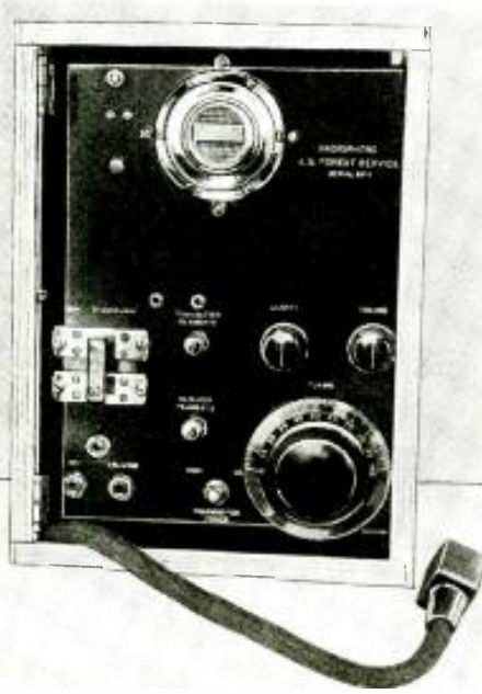
PORTABLE RADIO TELEPHONE To aid "smoke chasers" in their work. (Photo. Dept. of Agriculture)
